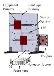
Fig. 3. Satellite Structural Panel demonstrator with attached test coupon (3D-model including fiber optic sensor systems
