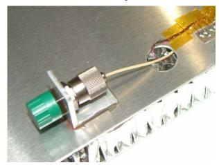
Fig. 6. Sensor fiber interface and FO connector
