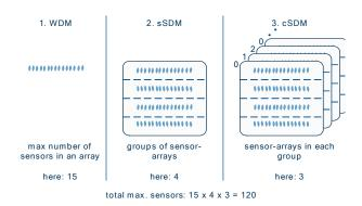
Fig. 9. Combination of spatial and wavelength division multiplexing
