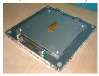
Fig. 5. Smart Panel Test coupon for verification of MAIT, functional and environmental testing
