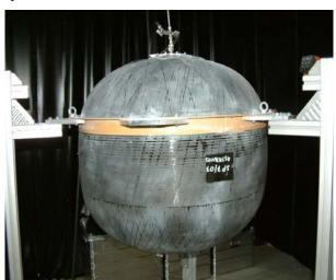
Fig. 7. Satellite Fuel Tank demonstrator
