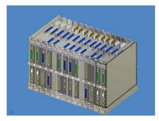
Fig. 10. Potential position of Interrogator Unit in a standard On-Board Computer (OBC) from Astrium
