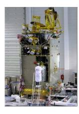
Fig. 1. Picture of Inmarsat 4 & Intelsat X satellite based on the Eurostar 3000 platform
