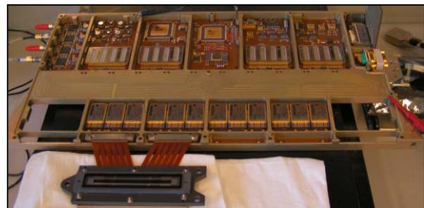
Fig. 8. View of a Video Unit Board coupled with a CCD module during electrical tests.
