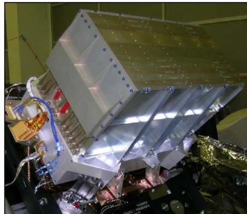
Fig. 7 View of the Video Unit fully integrated on its dedicated mechanical support ready for EMC environment tests.
