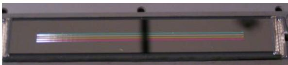
Fig. 5 View of stripped multispectral filters glued on CCD AT 71554
