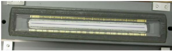
Fig. 3. View of PAN CCD 98-50
