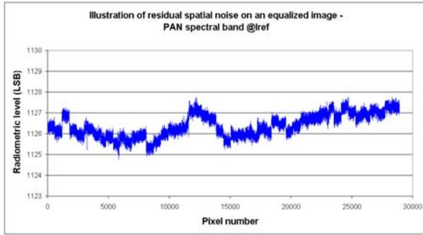
Fig. 16. PAN Image after equalization @ Iref
