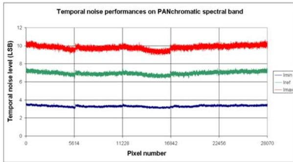
Fig. 11. Temporal noise on PAN spectral band (exc. inter-CCD areas)
