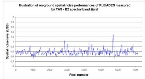
Fig. 17. Spatial noise @ Iref on B2 spectral band
