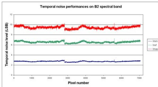
Fig. 12. Temporal noise on B2 spectral band (exc. inter-CCD areas)
