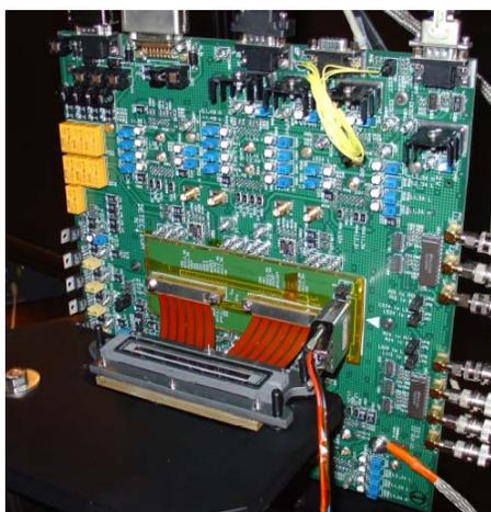
Fig. 2. View of equipped CCD module under electrical tests with Thales Alenia Space specific electrical interface board.
