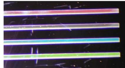
Fig. 6. View of optical coatings used on stripped multispectral filters
