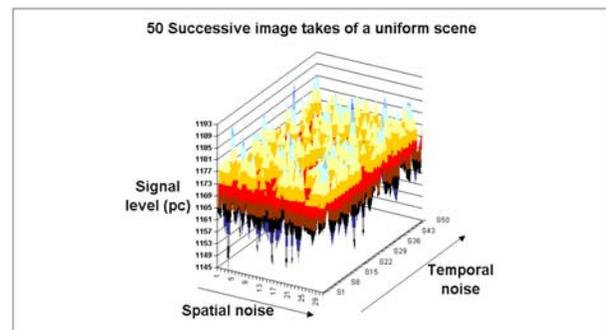
Fig. 10. Example of successive PANchromatic images of a uniform scene
