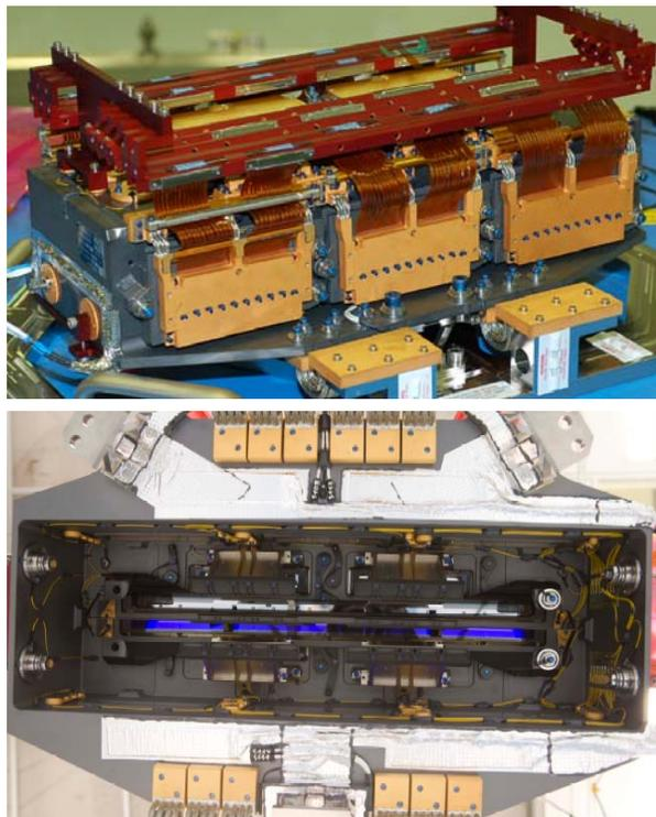
Fig. 1. Views of the PLEIADES Focal Plane Assembly (top and bottom faces)
