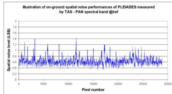
Fig. 18. Spatial noise @ Iref on PAN spectral band
