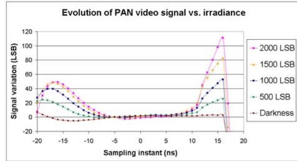
Fig. 9. Example of PANchromatic video signal
