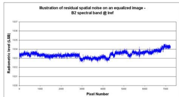
Fig. 15. B2 Image after equalization @ Iref
