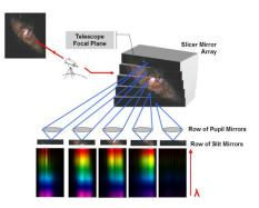
Figure 3: Image slicer principle
