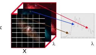
Figure 2: 3D spectroscopy illustration.
