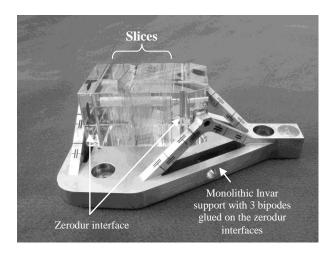
Figure 4: image of a block of slicers
