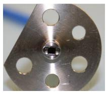
Fig. 3. a) LOLA optical fiber array to fan out assembly, b) 200X magnification end face image of optical fiber array, c) the LOLA custom adapter interface to the receiver optics.
