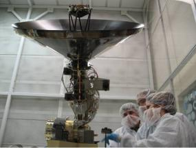
Fig. 13. a) The team investigates - the full motion of the High Gain Antenna comes close to the optical cable routing configuration.
