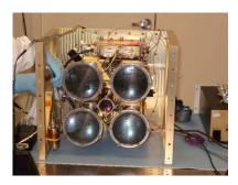
Fig. 1. The Mercury Laser Altimeter consisted of four telescopes with fiber coupled from each to four individual detectors.[6]
