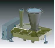
Fig. 2. a) Artistic rendition of the LRO with the High Gain Antenna pointing at the earth while instrument LOLA is viewing the moon's surface, b) Artist's rendition of LOLA.
