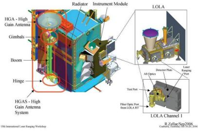
Fig. 8. Details on the LRO Optical Fiber Link Path from the LRT to LOLA, D. Smith [12]
