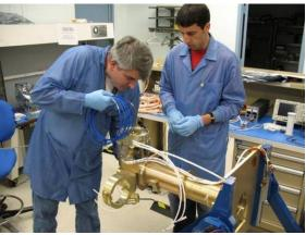
Fig. 11. a) FOB 2 being routed into the cable wrap on gimbal 2, b) Photonics Group members, Richard Chuska and Robert Switzer work on integration of the FOBs to the gimbal cable wraps.
