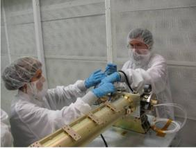
Fig. 12. a) Richard Chuska and Melanie Ott conduct transmission testing on FOB 2 with gimbals now attached to the entire boom arm, b) Melanie Ott and Adam Matuzseski integrate the FOB 2 to a safe position after integration down the boom, while awaiting the mandrel installation.
