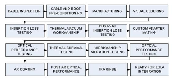
Fig. 4. LOLA Optical Fiber Bundle Array Assembly Delivery Flow
