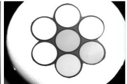
Fig. 9. a) Example of a LR seven fiber optical assembly, b) endface picture of Diamond ferrule at 200X magnification with 7 440 micron outer diameter optical fibers packed precisely together to minimize the epoxy bond line.
