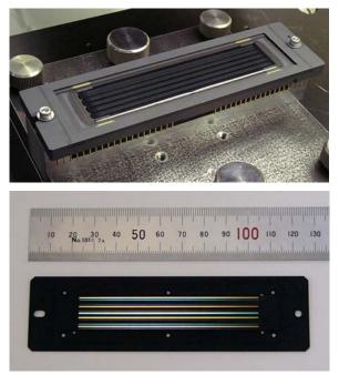
Fig. 4 11 line CCD and bandpass filter assembly
