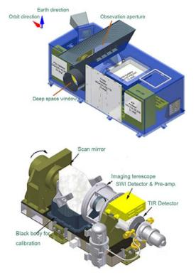
Fig. 3 IRS instrument 3D draw and its inner configuration
