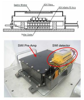
Fig. 5 SWI detectors cross-section drawing and SWI detection unit
