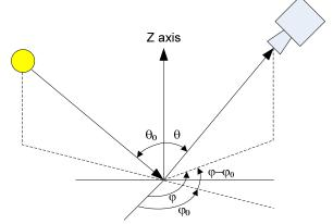
Figure 1. Illumination geometry of a planetary body
