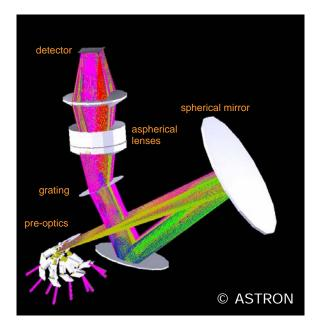
Figure 4. SPEX instrument baseline optical design
