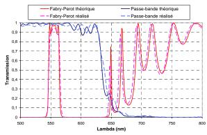
Fig. 5. Comparison between theoretical and measured spectral responses
