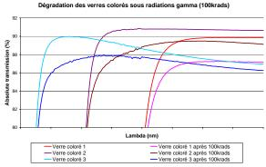
Fig. 7. Degradation of coloured glasses under Gamma radiations
