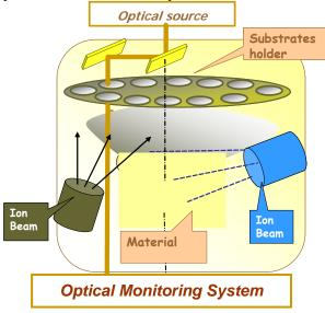
Fig. 4. Dual Ion Beam Sputtering principle
