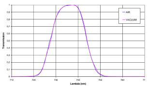
Fig. 8. Spectral measurement under normal atmosphere and in vacuum
