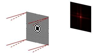
Figure 1: Image formation by a Fresnel Array. Here, a double point source is imaged by an orthogonal geometry one.
