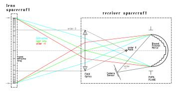
Figure 3: Synoptic diagram of an achromatized Fresnel Diffractive Imager. In the ultra-violet domain ( $\lambda < 250 \rm nm$ ), a blazed Fresnel Mirror plays the major role in the chromatism correction scheme.
