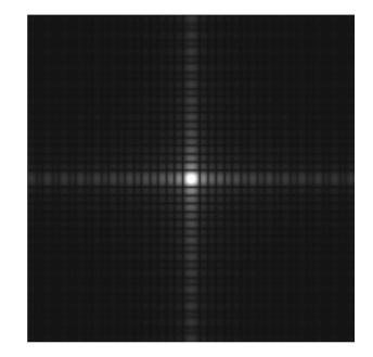
Figure 2: Example of Point Spread Function of an apodized Fresnel Diffractive Array. The brightness scale has been strongly flattened for display, to reveal the faint residual light in the four quadrants of the field.
