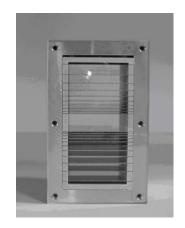
Fig. 14. Test module for tests performance of glass foils vs. shaped Si wafers. Test elliptical Kirkpatrick-Baez optical system, focus 0.5 m,  $58 \times 50 \times 100 \text{ mm}$ , glass foils  $40 \times 40 \times 0.3 \text{ mm}$ , Si wafers  $40 \times 40 \times 0.4 \text{ mm}$ .
