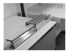
Fig. 15: Test parabolic KB X-ray imaging system based on parabolically shaped glass foils with dimensions of  $300 \times 100 \times 0.3$  mm. The complete KB
