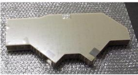
Fig. 2 Picture of the Base-plate built for the Aladin Mie Spectrometer
