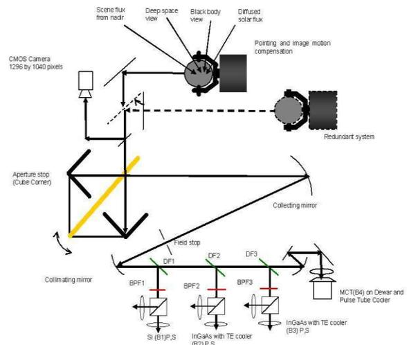
Fig.5 TANSO-FTS Optical Schematics
