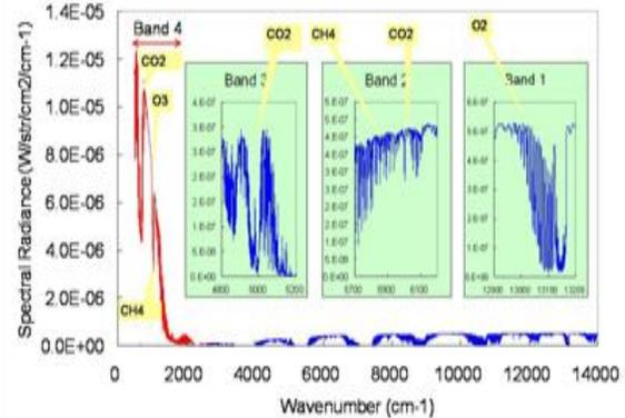
Fig. 4 TANSO-FTS Spectral Coverage and observed gases
