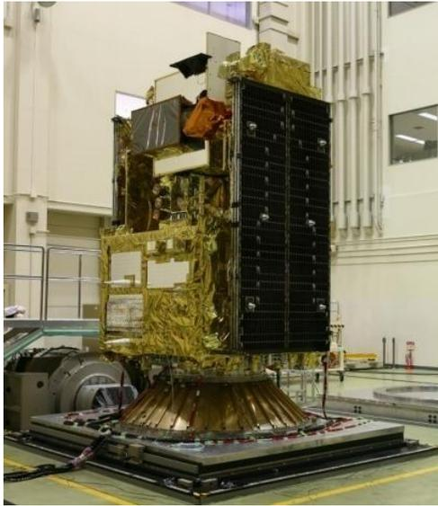
Fig. 2 GOSAT PFM under vibration test
