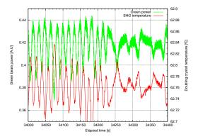
Figure 5: Time evolutions of green beam power and doubling crystal temperature.
