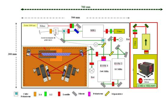
Figure 6: Experimental layout of the laser stabilization with iodine in cavity.
