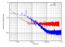
Figure 4: Temperature stabilities of the cell cold finger and doubling crystal (improved feedback electronics).
