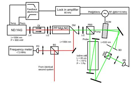
Figure 1: Experimental layout of the iodine laser stabilization.
