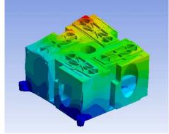
Figure 5 First mode of Natural frequency. This picture shows a torsion movement around one of the mounting points.
