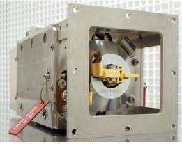
Fig. 5. Flight model sorption cooler of the HERSCHEL Satellite
