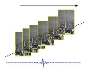
Fig. 6. The interferogram along the diagonal, the arrow is the direction of movement .
