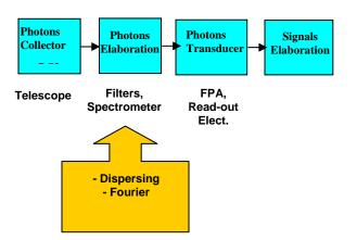
Fig. 1. Imaging Spectrometer Blocks Diagrams
