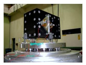
[Figure 8] RV Test of Structure Model
