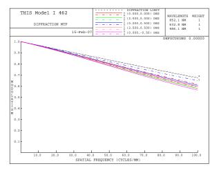
[Figure 4] MTF Analysis of TIS Telescope
