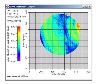
[Figure 11] Measurement of Wavefront error at the edge
