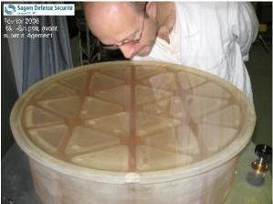
Fig. 9 SAGEM second breadboard after rough machining
