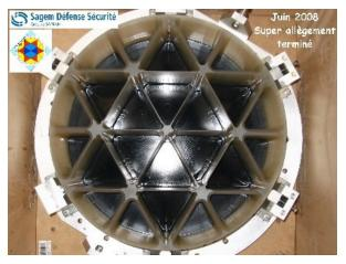
Fig. 10 SAGEM second breadboard after final machining (12 central cells only)
