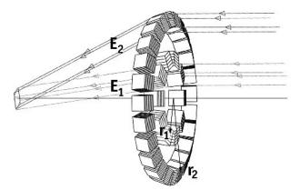
Fig 1 : Principle of a Laue lens : crystals disposed in concentric rings diffracts radiations coming from infinity towards a common focus.
