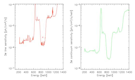
Figure 5 : Narrow line (left panel) and continuum (right panel) sensitivity of GRI telescope in the energy band covered by the Laue lens. These calculations assume 100 ks of exposure time, and an energy bin of E/2 for the continuum sensitivity. On the left panel, the cross shows the sensitivity for the 847 keV broadened line.
