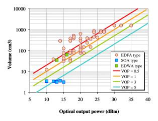
Figure 5: Comparative volumic optical power (VOP) of OA products
