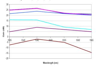
Figure 6: Gamma radiation-induced degradation of spectral gain
