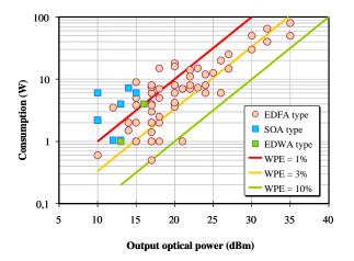
Figure 4: Comparative wall-plug efficiency (WPE) of OA products
