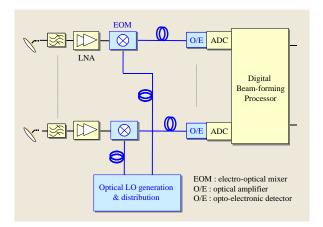
Figure 2: Advanced receive antenna with opticallyassisted digital beam-forming
