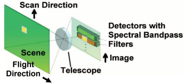
Figure 2: In-field separation of spectral channels. Due to the satellite motion, the image of a certain pixel moves straight over the focal plane with an arrangement of detectors. There it is sequentially imaged by detectors with different spectral filters.
