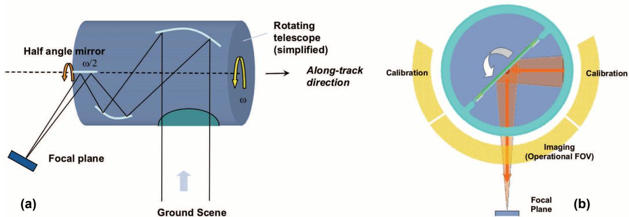
Fig. 1: (a) Simplified principle of a rotating telescope scanner. The off-axis telescope rotates around an axis perpendicular to the viewing direction. A stationary image in the focal plane is produced by the plane "half-angle mirror", which rotates at half the rate. (b) Different portions of the field-of-view (FOV) are used for imaging and calibration, without need for additional mechanisms to move calibration sources into the optical path or interruption of normal operation.
