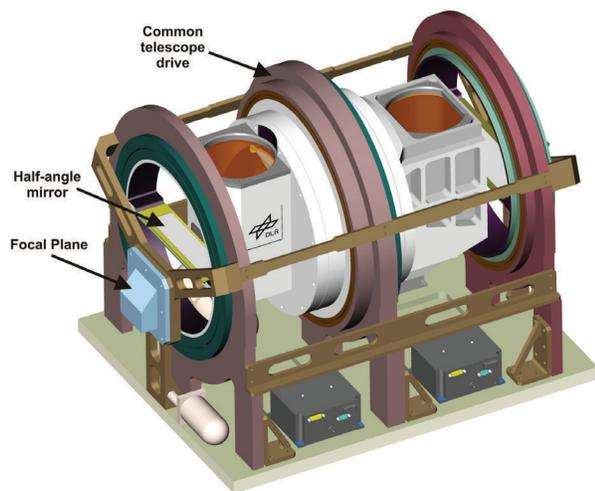
Figure 5: Design of a METimage instrument with visible and infrared light processed separately (METimage version C), therefore with two apertures. A common structure and common telescope drive provide good synchronisation and a compact design.
