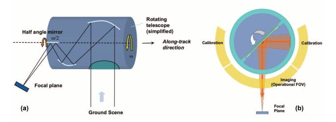
Fig. 1: (a) Simplified principle of a rotating telescope scanner. The off-axis telescope rotates around an axis perpendicular to the viewing direction. A stationary image in the focal plane is produced by the plane "half-angle mirror", which rotates at half the rate. (b) Different portions of the field-of-view (FOV) are used for imaging and calibration, without need for additional mechanisms to move calibration sources into the optical path or interruption of normal operation.
