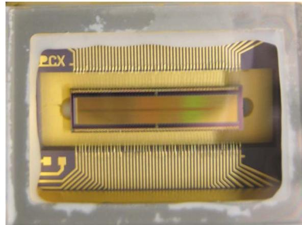
Fig. 3. Photo of the PMDG sample within its package.
