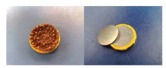
Fig. 7: Problems during coating development (left: unexpected Cu growth, right: poor adhesion)
