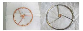
Fig. 8: M2 Manufacturing Steps: Left: raw part Cu plated, right: final raw part
