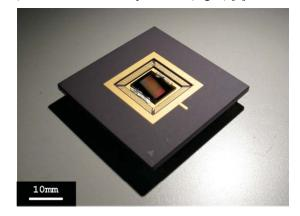
Figure 1. 64 x 32 micromirror array with high fill factor in the vertical direction provinding long slits. Each mirror measures  $200 \times 100 \ \mu\text{m}^2$ .Two wafer level bonding steps are required to process these arrays.
