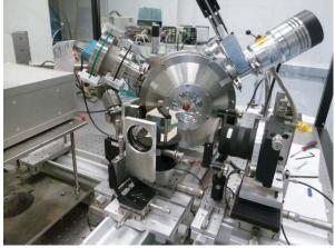
Figure 2. Cryogenic chamber installed on our interferometric setup. MMA with 64 x 32 micromirrors is integrated (100 x 200  $\mu$ m<sup>2</sup> micromirrors).
