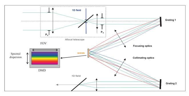
Figure 9. Function F5: Spectral selection, large FOV programmable spectrograph
