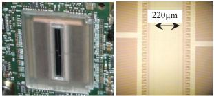
Figure 4. PMDG components by SLM, whole device picture and detail of the ribbons (length 220µm).
