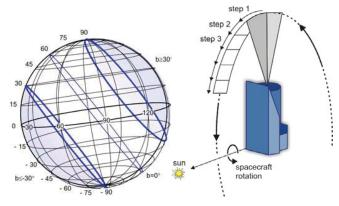
Fig. 2 Extragalactic sky survey geometry in ecliptic coordinates (left) and step & stare sky survey principle (right).
