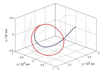
Fig. 3 EUCLID mission reference orbit. The period until the last transfer correction manoeuvre is indicated by blue color.
