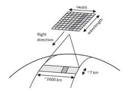
Figure 2. TROPOMI measurement principle
