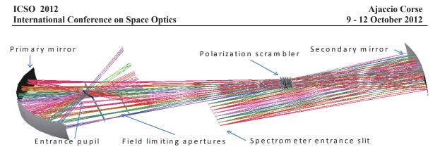
Figure 3. 3D view of TROPOMI telescope
