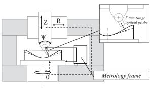
Figure 6. NANOMEFOS machine concept with long range optical probe and separate metrology frame
