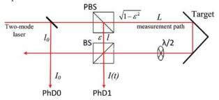
Figure 1. Schematic diagram of the telemeter
