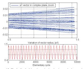
Figure 15. The "spikes" of the telemetric signal trajectory in the complex plane when the measurement path length is varied by 25 $\lambda$ opt  $\approx$  39  $\mu$ m in 10 mn
