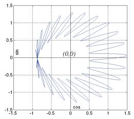
Figure 3. The calculated two-mode interference pattern obtained, at constant  $v_{oot}$ , when the target is moved continuously over  $\Lambda/2$ , with  $\varepsilon = 0.25$
