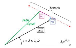
Figure 2. Addition, in the complex plane, of the three contributions to the PhD1 two-mode interference, signal. The phase  $e^{il_0\delta/c}$ , of the PhD0 photodiode, is taken as the phase reference.
