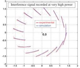
Figure 10. Spikes recorded at very high power, for different position of the target: complex plane representation. The optical frequency is kept constant. Blue data: simulation, with  $\varepsilon = 0.22$ , taking into account the AM-to-PM and saturation effects
