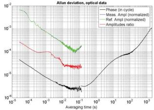
Figure 11. Stabilities of the relative phase and amplitude ratio measurements with an optical signal without interference (the reference path is masked). The average acquisition rate is 27µs. Points "Ampl C1" are almost completely covered by points "Ampl C2".
