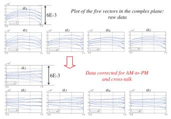
Figure 9. Spikes recorded by scanning the measurement length *L*, without and with AM/PM effect correction
