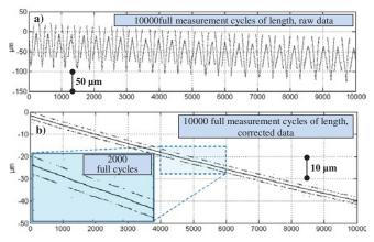
Figure 16. The result of 10,000 full cycles (a) without and (b) with correction for electronic distortions. For convenience, the length values are shifted by 7, 492717m
