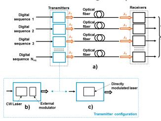
Figure 1. a) Link configuration including  $N_{sq}$  transmission channel; b) and c) are two options of the transmitter configuration.
