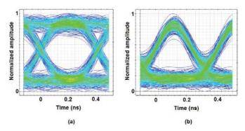
Figure 5. Eye diagram for BR = 2.5 Gb/s and DFB laser power = 3.3 dBm, in case of either NRZ encoding (a) or RZ encoding (b).
