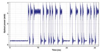
Figure 3. Time dependence of the DFB laser output. Laser power = 5 dBm.
