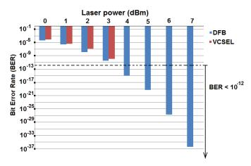
Figure 4. Bit error rate when a VCSEL or a DFB laser is utilized for the digital transmission.
