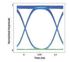
Figure 6. Eye diagram for BR = 2.5 Gb/s and DFB laser power = 3.3 dBm, in case of RZ encoding.
