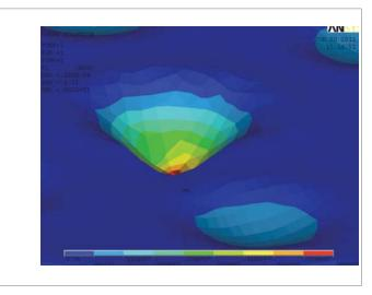
Fig. 9. The tensile stress (s1) in the glass, the maximum stress is about 6 MPa and remains below the admissible value for Zerodur, fixed at 30 MPa.
