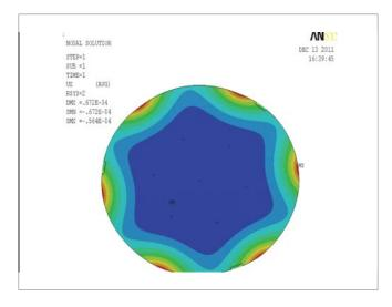
Fig. 7. . Displacements due to the flexure system for  $10^\circ C$  temperature variations. The PTV is about 11 micron.
