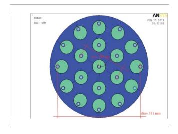
Fig. 4. The new proposed actuator pattern and the diameters of the two reference rings
