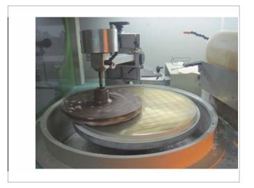
Fig. 5. Zerodur blank during polishing step
