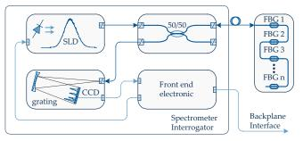
Figure 5: Fiber-optic interrogator based on a spectrometer and a broad-band light source.
