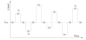
Figure 7: Measurement cycles for a scan through the lasers spectrum. Each wavelength ( $\lambda_1$  to  $\lambda_n$ ) is set up from the same mid-wavelength to identify long term drifts.
