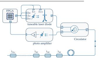
Figure 4: Fiber-optic interrogator based on a tunable laser with control FPGA, optical circulator, FBG sensors and photodiode.
