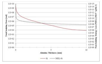
Figure 2: Total Ionizing Dose (TID) for silicium and non-ionizing energy loss (NIEL) in dependence of aluminum shielding thickness for the H2-Sat mission with a duration of 15 years in geostationary orbit [2].
