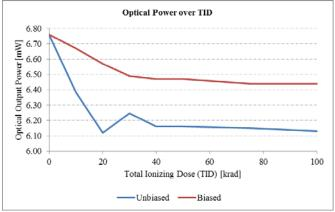
Figure 9: Optical output power for the biased (red curve) and unbiased (blue curve) laser diode respectively over TID.
