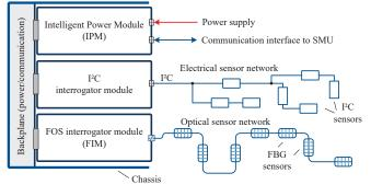
Figure 1: Concept of the HSB system with Intelligent Power Module (IPM), I<sup>2</sup>C Interrogator Module (IIM) and Fiber-Optic Interrogator Module (FIM).
