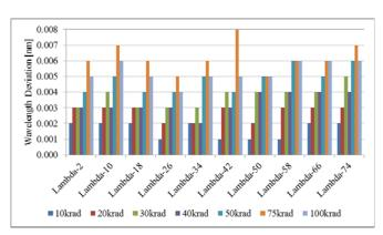
Figure 10: Wavelength deviation of different wavelengths from their original setup wavelengths at different TID levels. The maximum deviation reaches 8 pm.
