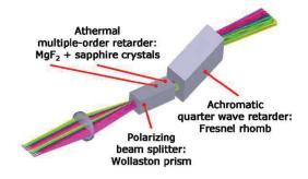
Fig. 1: Optical configuration for the polarization encoding system.
