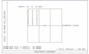
Fig. 6: Footprint diagram at detector for one arm configuration consisting of 5 viewing directions. Each arm is imaged onto one detector compartment to reach a total of 30 viewing directions.
