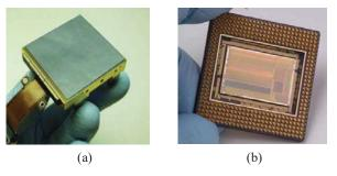
Fig. 4: (a) Teledyne H2RG detector; (b) Teledyne SIDECAR ASIC
