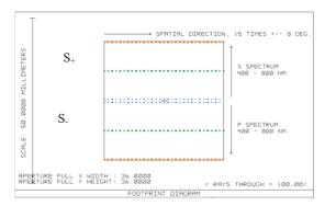
Fig. 3: Footprint diagram at detector indicating both  $S_+$  and  $S_-$  polarisations in the spectral direction. In the spatial direction a 16° swath is imaged 15 times. For each of the 15<sup>th</sup> viewing directions three field points are indicated: one on-axis and two at the edges of the field ( $\pm 8^\circ$ ).
