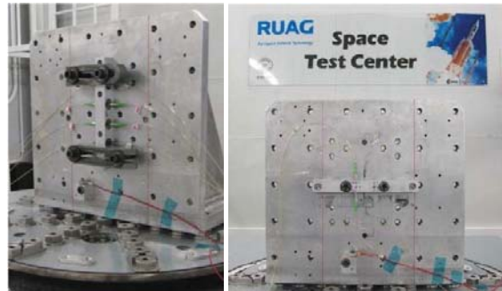
fig. 9 Vibration table at Ruag Space
