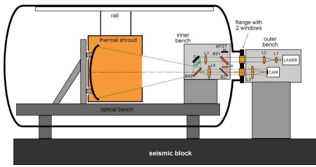
Figure 7. Configuration of the thermal vacuum test.
