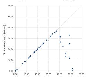
Commercial interferometer measurements (arsec) Figure 6. Comparison of the rotation angle measured by the new instrument and the Doppler effect interferometer.
