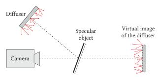
Figure 1. Observation of speckle from a specular object.
