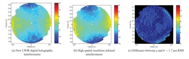
Figure 9. Comparison of the deformation of the reflector for the same temperature variation with a previous results obtained on the same reflector with a high spatial resolution infrared interferometer.
