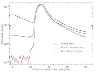
Figure 10. Impact of the vanes on the stray light reduction performance.
