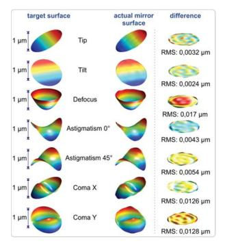
Fig. 11 Comparison between the target mirror surface and the actual mirror surface along with the residual surface error
