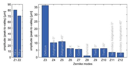
Fig. 7 Numerically calculated low order Zernike-amplitudes for the presented mirror configuration
