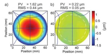
Fig. 3 Initial deformation of the coated glass substrate a) total deformation b) residual deformation at best defocus
