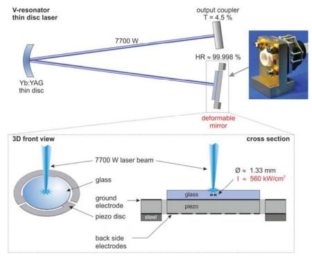
Fig. 12 Experimental setup to verify the power handling capability of the deformable mirror
