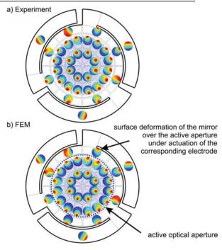
Fig. 9 Influence functions of the mirror electrodes. Shown is the deformation that results if a single electrode is supplied with a voltage of 100 V. The false-color elevation plots representing the mirror deformations are plotted at the position corresponding to the activated electrode. a) Experimentally measured deformations,
