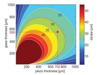
Fig. 6 Defocus stroke of the laminate as a function of individual layer thickness for an applied voltage of 400 V
