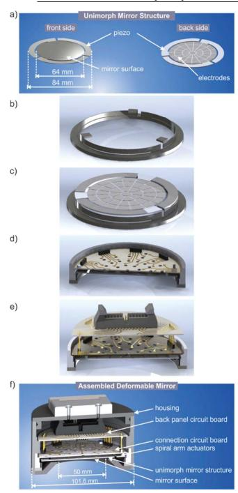
Fig. 4 a) unimorph mirror structure, b) mounting ring, c) mounted mirror structure, d) connection board on top of the mirror back side, e) back panel circuit board on top of the connection board, f) cross-sectional view of the assembled mirror
