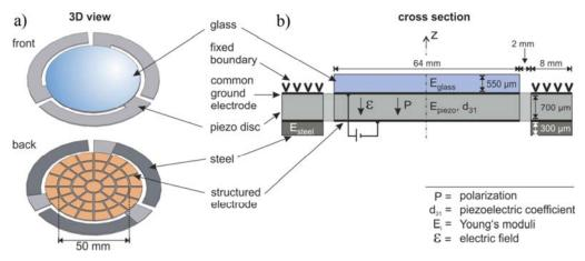
Fig. 1 a) Three-dimensional view of the deformable mirror along with the electrode pattern b) Cross-sectional view
