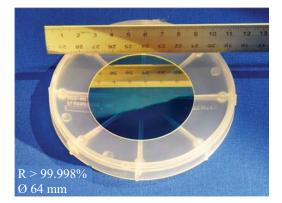
Fig. 2 HR-coated glass substrate (R > 99.998% @ 1030 nm)
