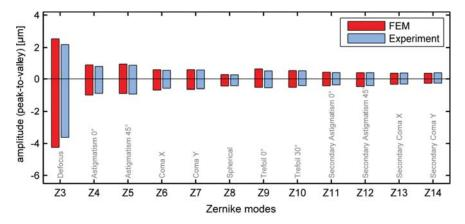
Fig. 10 Comparison between calculated and measured Zernike amplitudes generated by the smallersized prototype mirror
