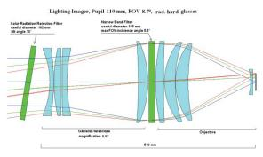
Figure 5 - Single optical channel layout with Galileian telescope
