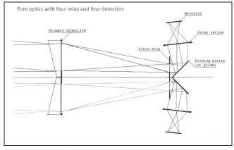
Figure 11 - single primary with four relay approach
