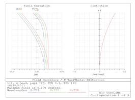
Figure 21: distortion and field curvature
