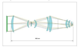
Figure 14: Dioptric with relay optical layout
