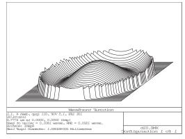
Figure 18: On axis RMS wavefront error function
