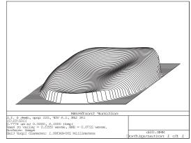
Figure 19: maximum FOV RMS wavefront error function
