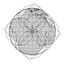
Figure 3 - LI coverage with 4 Optical Channel concept
