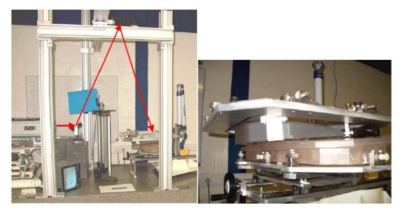
Fig.4. Primary mirror test bench
