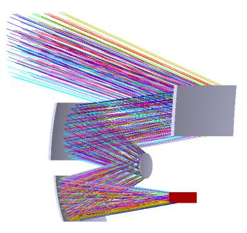
**Fig.1.** Four-mirror optical lay-out Proc. of SPIE Vol. 10565 105650C-3
