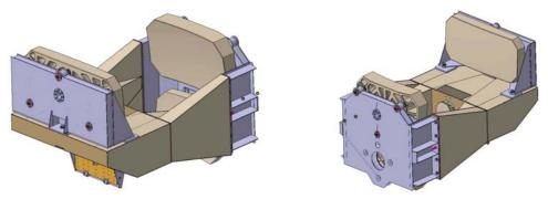
Fig. 3. Telescope opto-mechanical concept view
