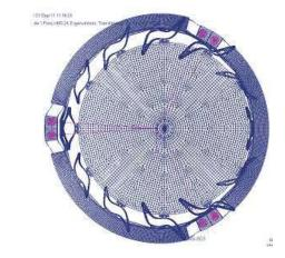
Figure 3. FEM analysis : first Eigenfrequency in radial direction higher than 400 Hz
