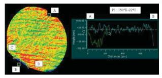
Figure 13. Raw WFE measured at 150 K. Edge effect are visible. The cuts are given for both directions [AB] and [CD]. Measured deformation in local pantograph area is 180 nm PTV
