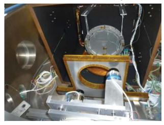
Figure 8. Breadboard in its vaccum chamber for optical tests
