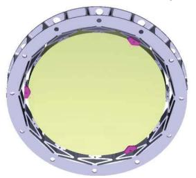
Figure 2. Mechanical concept proposed for large lens in cooled environment
