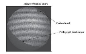
Figure 10. Exemple of fringes obtained on P1 position in vacuum and in cold temperature
