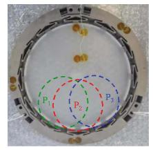
Figure 9. Measurement at 3 sub pupils level (P1, P2 and P3) in order to point out the edge deformation
