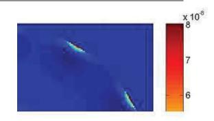
Figure 14. Predicted deformation at 150 K due to the pantograph interface. Mechanical surface deformation is calculated around 80 nm PTV which is equivalent to WFE for reflected light of 160 nm.
