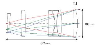
Figure 1. Optical Thales Alenia Space design for PLATO mission
