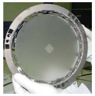
Figure 5. Scale 1 breadboard design for space applications. A centered mark is accommodated to ease the WFE exploitation.
