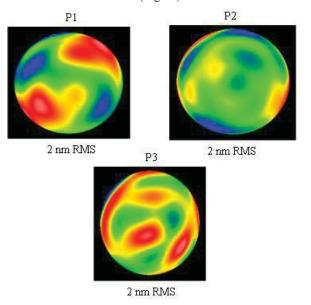
Figure 15. Differences between both reference mesurements (at ambient) before the test sequence and after. Analysis performed for all scanned sub pupils (P1, P2 and P3).
