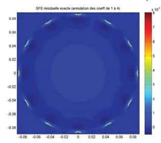
Figure 7. Prediction of the deformation between ambient and 150 K for the surface front error (SFE). The predicted WFE for the reflected beam equal to 2xSFE is lower than 10 nm RMS.
