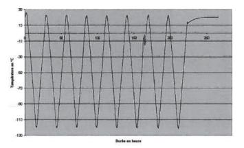
Figure 16. Thermal cycling successfully applied to the breadboard. Duration is in hours
