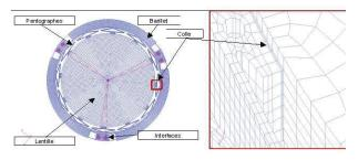
Figure 6. Breadboard precise FEM used for test predictions
