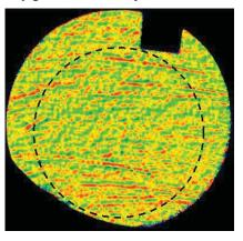
Figure 11. WFE difference between the reference (WFE measured at ambient) and the WFE at cold temperature (150 K here).
