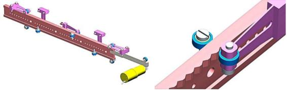
Figure 5 Design of the slit mechanism
