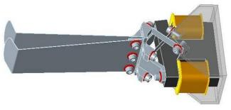
Figure 4 Design of the Cold Shutter
