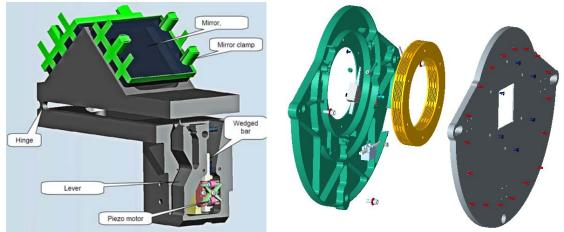
Figure 2 Left: Cryogenic Optical Path Difference correction mechanism. Right: Design of the Tip/tilt/focus mechanism. The mounting plate (turquoise) is placed right after the camera. Three motors control the distance and tip-tilt of the detector mounting plate (gray), while the spring (yellow) applies a necessary force on the motors to maintain the detector mounting plate in position.
