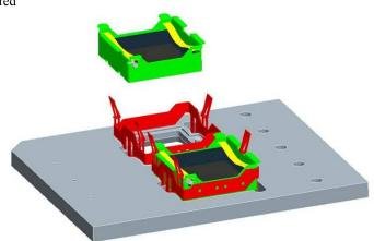
Figure 3 Mirror Clip design with the mounting structure (grey), the optical element (black), the mirror cell (green), leaf springs (yellow) and the cage (red).
