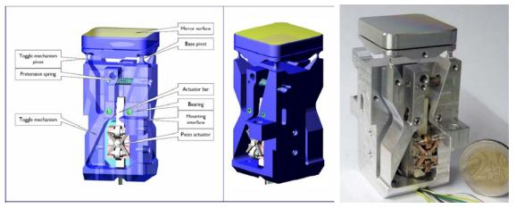
Figure 1 Tip-Tilt Mechanism including piezo motors
