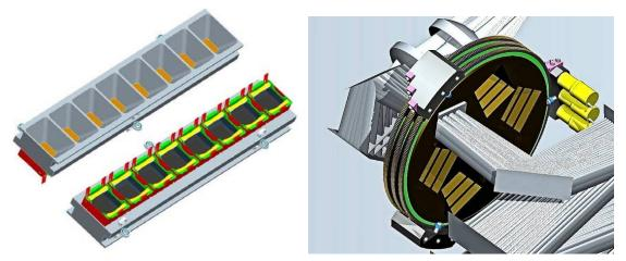
Figure 6 Left: Photometric slider using roller bearings. The figure shows front- and backside of the slider. Clearly visible are the mirror clips and the guiding ball bearings. Right: Design of 3 wheels with space for 6 optical components each.
