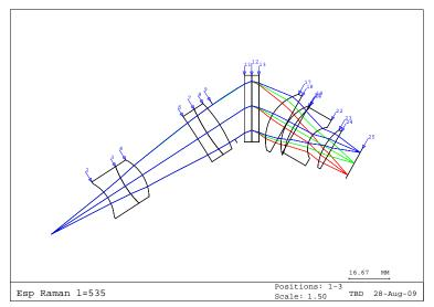
Fig. 5. Optical set-up of the spectrometer Proc. of SPIE Vol. 10565 105651E-5
