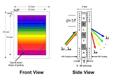
Fig. 2. Example of a VPH grating from Wasatch Photonics
