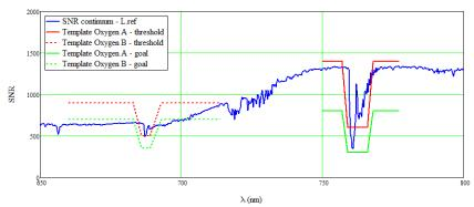
Figure 4 Calculated signal to noise ratio (SNR) for FIMAS with the assumptions: Dwell time 91 ms (slew down factor = 2), aperture size of 80 mm, SSD 300m and an instrument transmission of 0.2.
