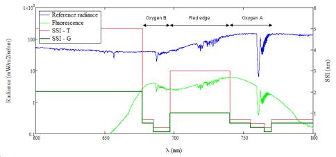
Figure 1 The plot shows the typical radiance received by the instrument, the contribution of the fluorescence signal (note the log-scale) and the requirement on the spectral sampling interval (SSI).
