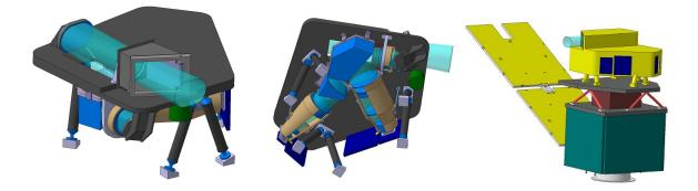
Figure 5 Example of FIMAS instrument configuration as seen from the top (left) and from the bottom (right). The optical concept from Figure 2 is easily recognized although the beam is folded here in order to keep the instrument within an acceptable volume. The most-right figure shows a possible accommodation of FIMAS on a MYRIADE platform.
