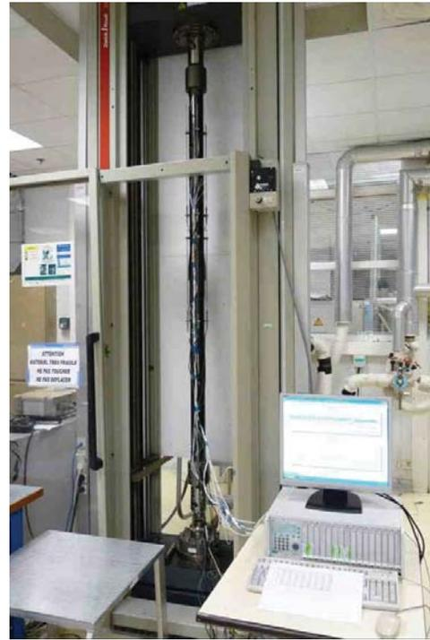
Figure III-7 2meter joined beams tested in tensile
