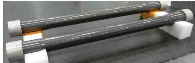
Figure III-4 qualification beams with polished surface and glued tests I/F
