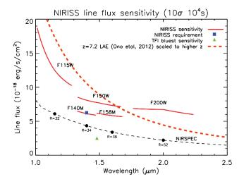
Fig.7. NIRISS sensitivity in WFSS mode.
