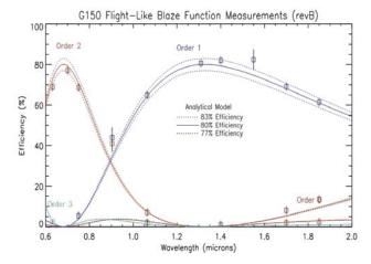
Fig.6. NIRISS GR150 grism efficiency curves, measured vs. modeled.
