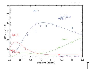
Fig.10. NIRISS G700XD efficiency, measured vs. modeled
