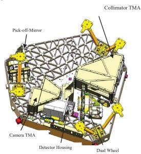
Fig.1. NIRISS Optical Bench configuration. Some baffles removed.
