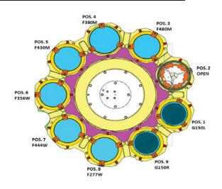
Fig.3. NIRISS filter wheel components
