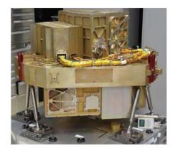
Fig.13. Fully assembled NIRISS (bottom) and FGS-Guider
