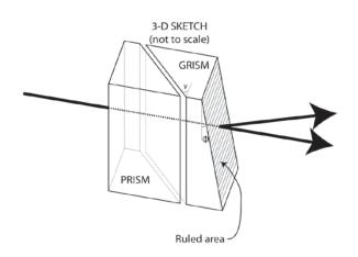
Fig.8. NIRISS GR700 grism -prism assembly
