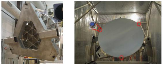
Fig.2. Primary mirror on his test support: on the left, view on the lightened part; on the right, view on the optical part, red circle indicates the position of the three reflectors balls
