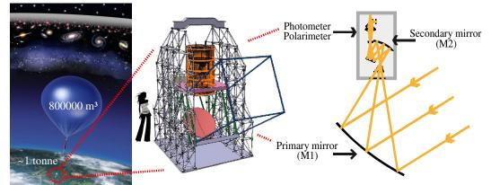
Fig.1. From left to right, a representation of the stratospheric balloon and onboard experiment, the instrument in the pointed payload, the optical concept
