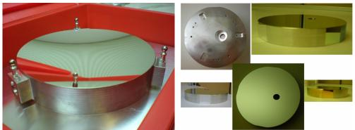
**Fig.5.** On the left, the secondary mirror with reference balls, on the right, the third mirror (the hole will be used for the internal calibration source)
