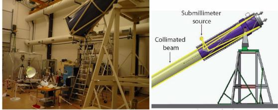
**Fig.3.** On the left, primary mirror under characterization; on the right, representation of the 1m diameter collimator and the incident submillimeter collimated beam (at an elevation angle of 30°)
