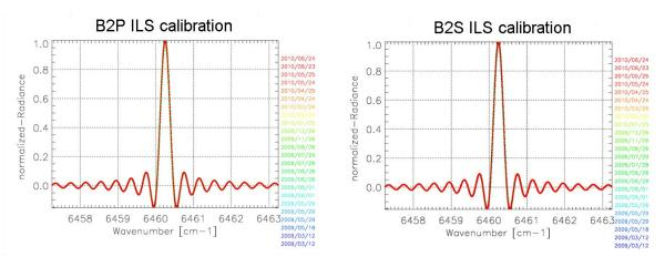
Fig. 5. ILS calibrations of Band 2 P and S by 1.55 micron on-board laser in one year Proc. of SPIE Vol. 10565 105651K-4
