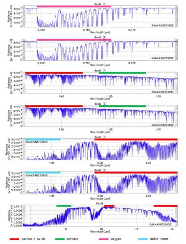
Fig. 2. TANSO-FTS spectral radiances observed over Tsukuba, Japan on April 23, 2009
