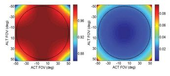
Figure 10. Typical example of polarisation sensitivity perofmances for a polarised (left) and a non-polarised (right) 3MI channel
