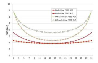
Figure 9. Spatial sampling distance variation across the filed of view of 3MI (red and green colours as of Fig. 4)
