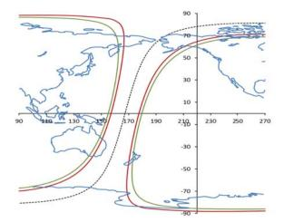
Figure 5. Yaw sterring ensures that the area scanned by the nadir view of the instrument is also covered by the other (off-nadir) views. The dark dotted line is the sub-satellite track.
