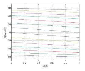
Figure 2. OZA sampling for targets on the sub-satellite track of 3MI (assumed ALT FOV =  $50.2^{\circ}$ )
