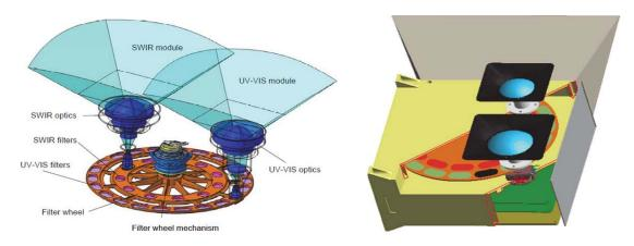
Figure 11. The 3MI instrument design concept (figures are from the Phase 0 studies)
