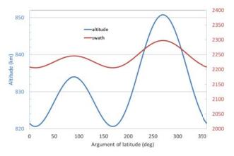
Figure 6. Variation of altitude and swath of 3MI along the MetOp-SG orbit
