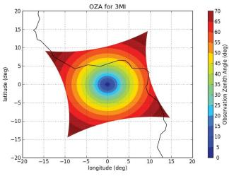
Figure 3. Footprint of 3MI VNIR channels
