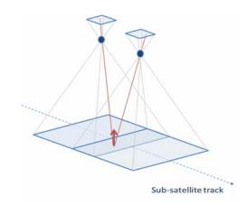
Figure 1. The 3MI measurement concept – This examples shows two images recorded in two along-track acquisition points
