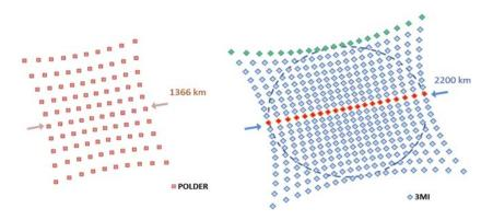
Figure 4. Comparison of the 3MI (right) and POLDER3 (left) footprints and swaths. Shown number of samples is only for visualisation.
