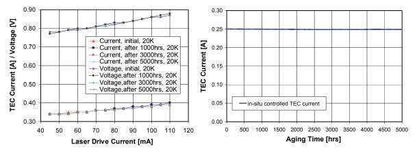
Fig. 6. TEC current and voltage at temperature difference of 20K vs. laser drive current (left diagram); in-situ monitoring of TEC current over aging, TEC temperature 40°C/case temperature 55°C (right diagram)
