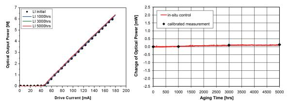
Fig. 5. LI-curves at Ohrs, 1000hrs, 3000hrs and 5000hrs aging (left diagram); change of in-situ controlled optical power (normalised) and calibrated optical power measurements over aging (right diagram)
