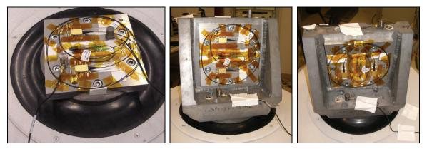
Fig. 4. LAT Vibration test setup, X-axis (left), Y-axis, Z-axis (right)
