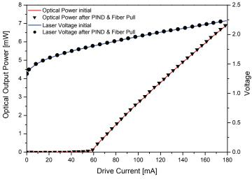
Fig. 3. LIV-characterization before and after PIND/Fiber Pull test
