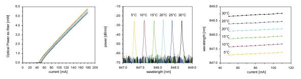
Fig. 2. LI-characteristics and spectra of a laser over temperature and drive current
