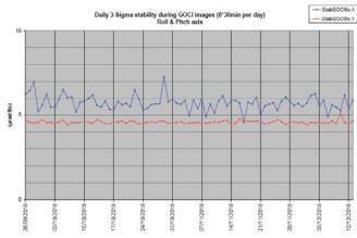
Fig. 13 : Typical LOS performance stability measured in orbit on COMS satellite
