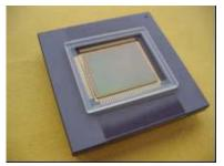
Fig. 6: GOCI CMOS Detector 2 Mpixels - 1415 x 1432 (shown with temporary window)
