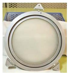
Fig. 12: Full pupil Solar Diffuser (external side)
