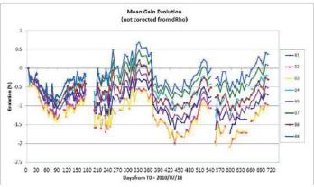
Fig. 18: Evolution of gain computed through GOCI in-orbit calibrations during the first 2 years.
