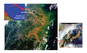
Fig. 15: Shangai Yangtze River, China, from raw data. The close-up on one slot shows streets detail (theoretical GOCI is resolution 500m at this latitude). An additional zoom shows the B8 pixels demonstrated the detection of sharp contrasts.
