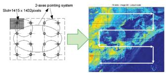
*Fig. 5: Principle of GOCI image acquisition* 32 Mpixels field of view is acquired in 16 slots
