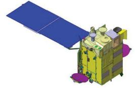
Fig. 1: COMS, in deployed configurations
