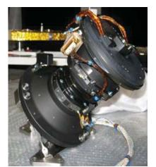
Fig. 7: GOCI Pointing Mechanism (w/o mirror)
