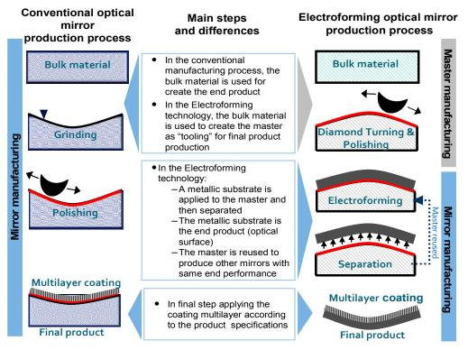
Fig. 2. Electroforming process
