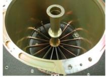
**Fig. 12.** Blocking shell and Mirror Interface Structure mounted on spider
