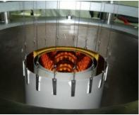
**Fig. 9**. Integration of Mirror Module with AVOB
