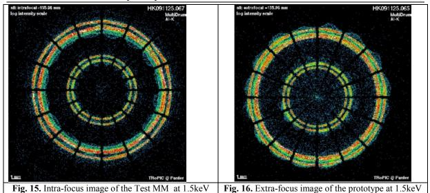
The image of the complete module is not only the result of the performance of the single shells but also dependent of an accurate alignment of all mirror shells. Here, all five foci are located within a circle of  $64 \mu m$  which is less than one detector pixel. The depth of the focus is within  $\pm 0.44 \ mm$ .
