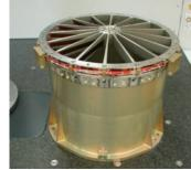
**Fig. 13.** Mirror module ready for shells integration
