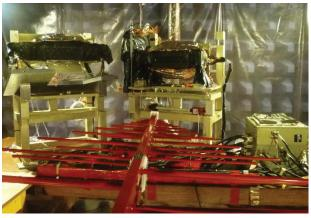
Figure 14: VNIR & SWIR EM FPAs during radiated EMC tests
