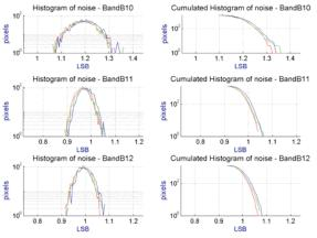
Figure 15: SWIR detector noise analysis during CS test (red and green: without injection, blue: with injection)
