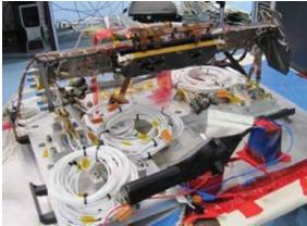
Figure 16: ESD test on VNIR FPA
