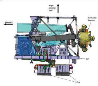
Figure 2: MSI mechanical architecture
